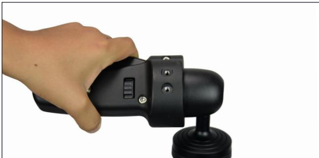
Replace the top plate as shown and secure tightly with the two screws.
