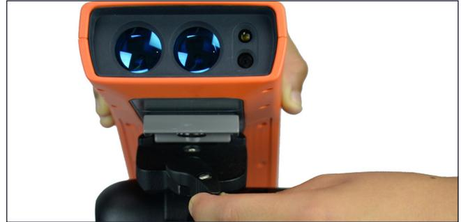
Lower the IKE unit into position and then turn the lever fully to lock the unit into place.
