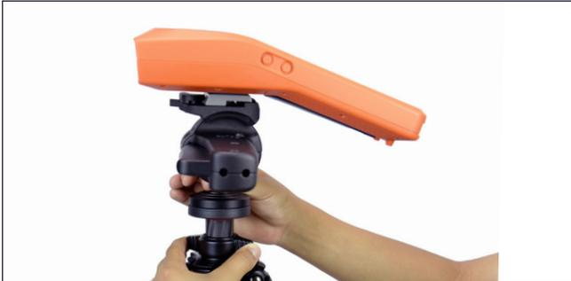
To adjust the position of the IKE device, with one hand hold the unit, and with your other hand squeeze the main lever and move to adjust.
