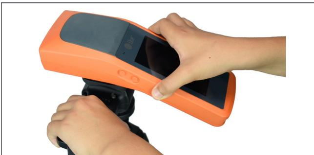
For span and pole height measuring, you can further tighten the movement of the lever so that the ball joint remains locked yet the pitch mechanism is still movable. To do this, while pressing the main lever with one hand, use your other hand to turn the friction dial and adjust the tension. Test the tension of the movement between adjustments.
